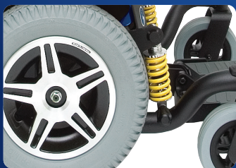
Active-Trac® ATX Suspension
