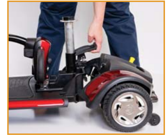
Step 4: Pull up on the drivetrain release lever to separate the front and rear frame sections!
